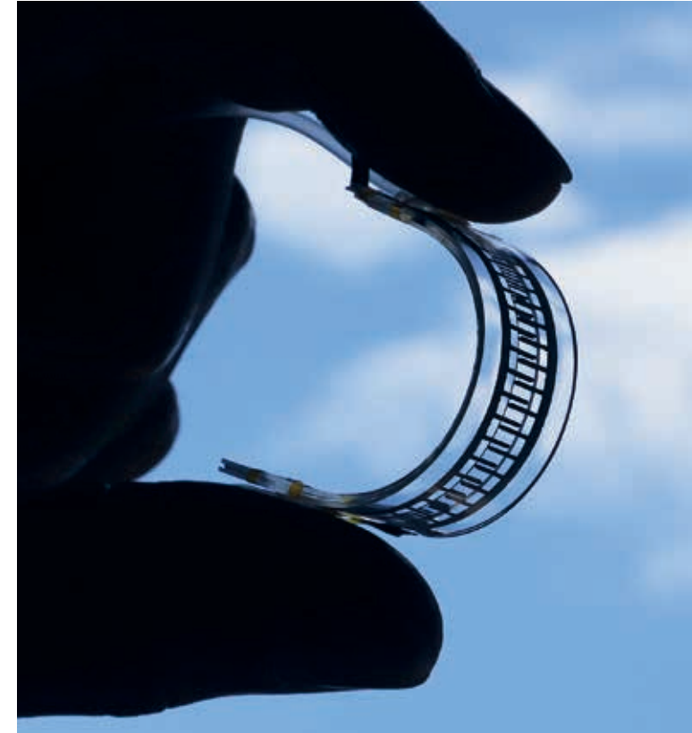
Stretchable pumps for Soft Machines. © Vito Cacucciolo and LMTS, EPFL 2019.
